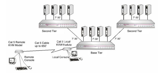
Figure 5 Two-Tier Configuration (with optional Remote Access)
